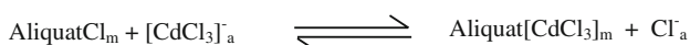
Fig. 3 Reaction between Aliquat 336 ion in the membrane (m) and trichlorocadmate in acid (a) solutions
